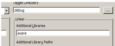
It is also possible to make use of either the Ecere runtime library, the Ecere Component Object Framework, or any eC shared library module by linking to it *statically*, that is to include the library within the executable file rather than as an external shared library. However, because the framework is oriented towards shared libraries, a shared library version of the module must first be built for the compiler to load module's available components.
